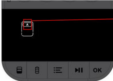
If P461 plug in Slot A, slot "A" icon flashing
