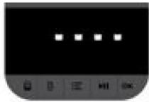
→ Plug in P461 (with batteries) into slot, LCD shows charging pack detection animation.
