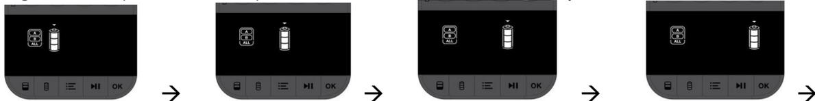
→ When detection done, LCD shows below and waiting user for battery selection.
