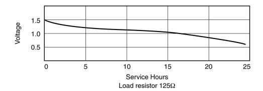
Average Service Capacity: 190mAh (rated capacity at  $470\Omega$  load, cut off voltage 0.9V at  $20^{\circ}$ C)
